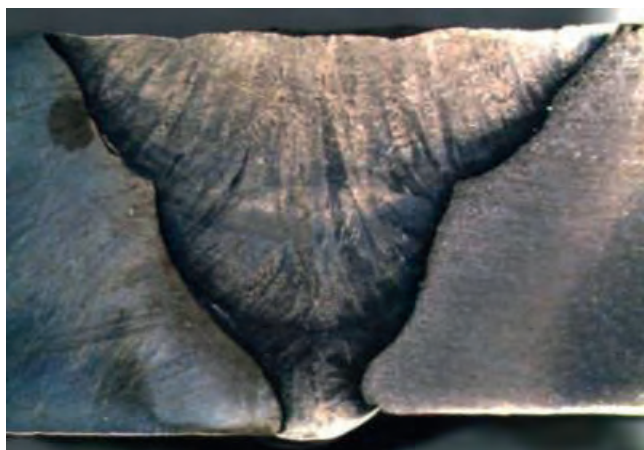
Figure 1. Anisotropic coarse-grain structure in austenitic materials.
