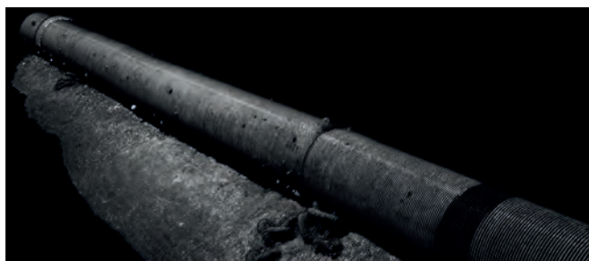
Figure 2. Pipeline 3D laser model captured with Voyis Insight Laser Scanner.
