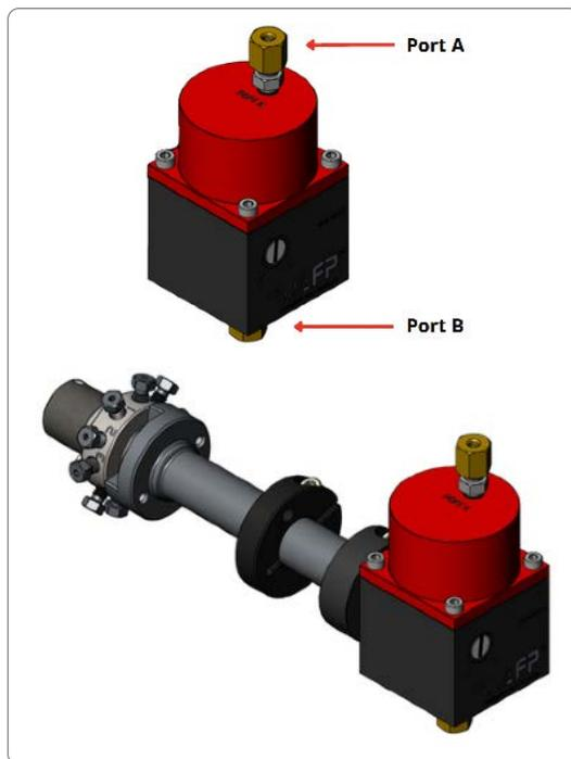
Various standoff assemblies can be used to mount the two-position rotary valves on the MPA. As a result, the user can isolate the actuator from the valve outside a heated area. AFP standoff assemblies come in 2", 3" and 4" lengths.
