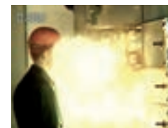
Pictures from test with TVOC. Arc fault without Arc Guard system.
