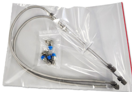
Figure 4.12: Picture of the optional PILATUS3 R 100K-M cooling vacuum feedthrough set with tubes through a standard DN40ISO-KF flange, and straight and elbow connectors for the detector head.
