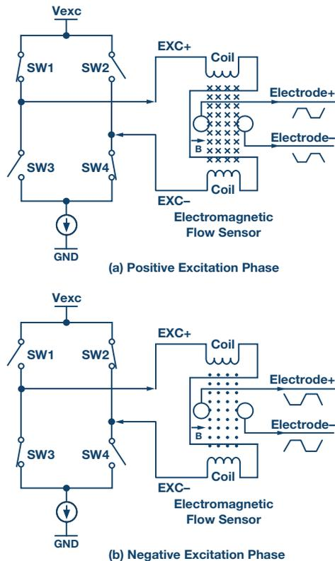
Figure 13. Magnetic field generation.
