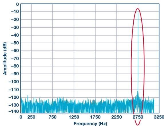
Figure 9. Alias when the ODR decimation sampling rate < twice the Nyquist frequency.
