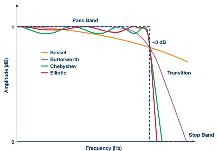
Figure 2. Ideal filter vs. practical filters amplitude response.
