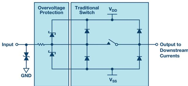
Figure 4. Traditional switch architecture with external discrete protection.
