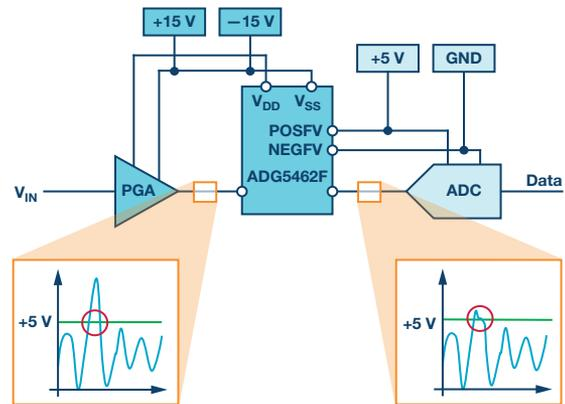
Figure 11. Data acquisition application example.
