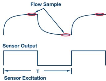
Figure 9. Flow signal sampling.
