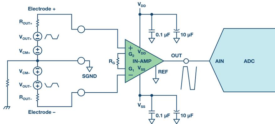
Figure 7. Common mode rejected by the preamplifier.
