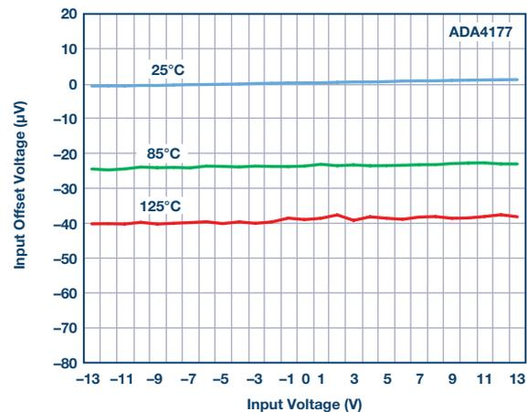
Figure 5. Input offset voltage vs. input voltage for ADA4177 with its integrated OVP.
