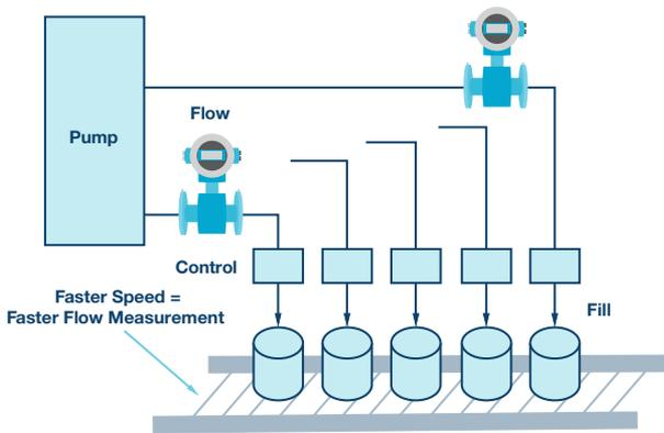
Figure 5. Liquid dosing/filling.
