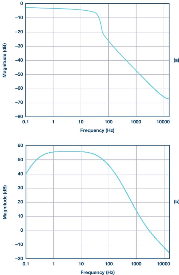
Figure 17. (a) Profile of a digital FIR low-pass filter. (b) Profile of an analog band-pass filter.
