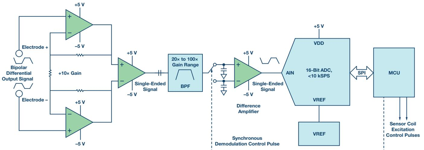
Figure 4. Traditional analog front-end approach.
