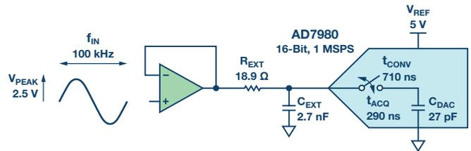
Figure 3. RC filter using AD7980 16-bit, 1 MSPS ADC.
