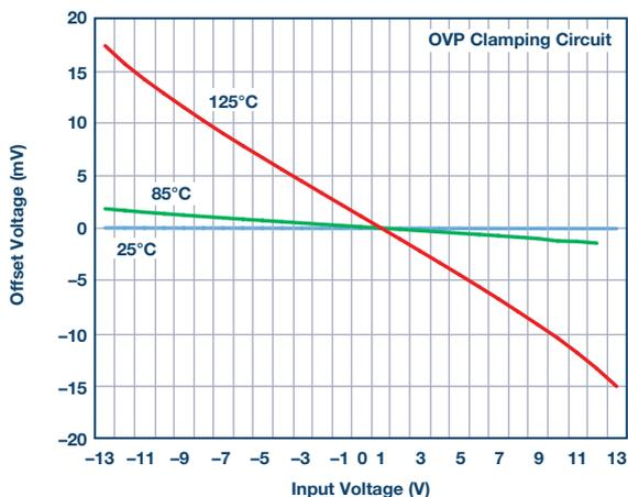
Figure 3. Input offset voltage vs. input voltage for an OVP clamping circuit added to ADA4077.
