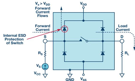
Figure 1. Overvoltage current path.
