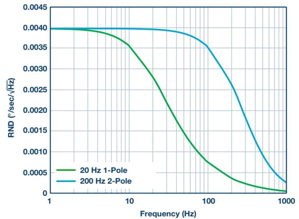
Figure 4. ADXRS290 noise density with filters.
