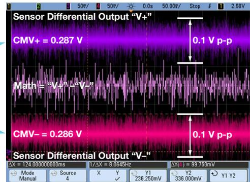
Figure 3. Output signal of electromagnetic flow sensor.
