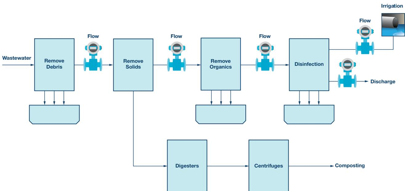
Figure 1. Simplified wastewater treatment plant.
