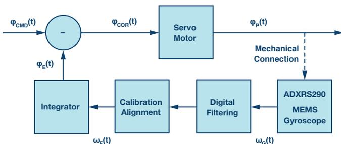
Figure 1. Example of a motion control system architecture.
