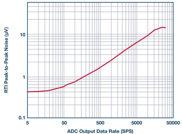
Figure 10. Test results of referred-to-input noise for oversampling architecture with AD8220 and AD7172-2.
