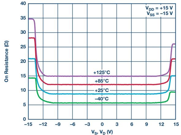
Figure 7. Fault protected switch on resistance.
