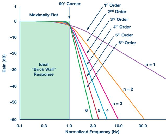
Figure 5. Ideal Butterworth filter transition band with different orders.
