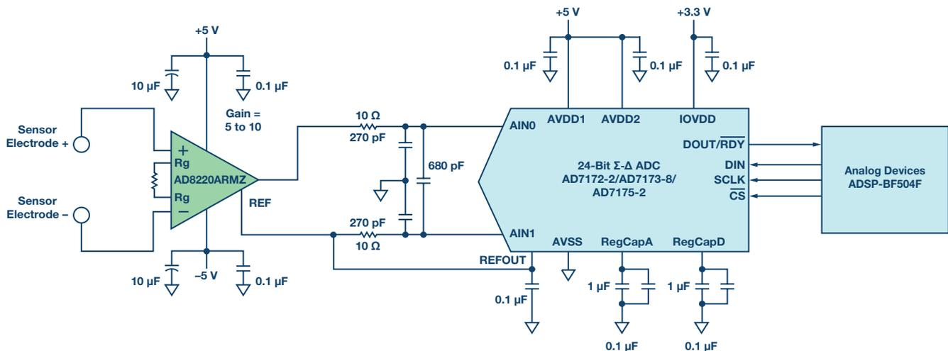
Figure 6. Oversampling architecture analog front end with AD8220 and AD717x-x.
