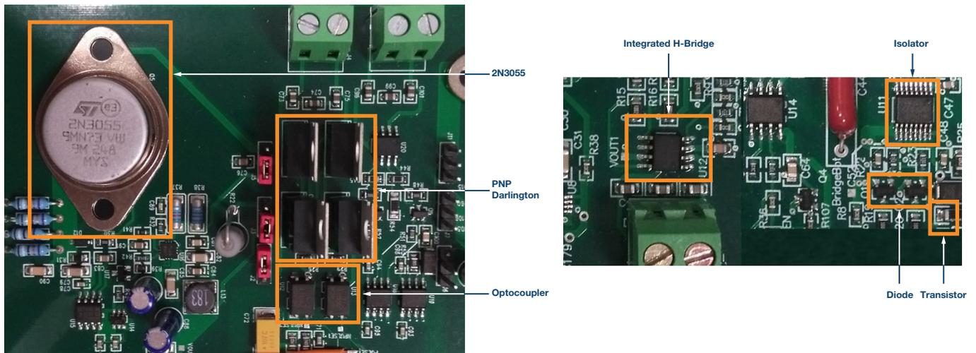
Figure 15. Area comparison of optocouplers vs. digital isolator design.
