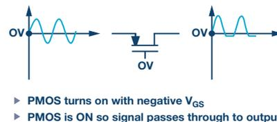
Figure 2. Overvoltage signal with power supply grounded.
