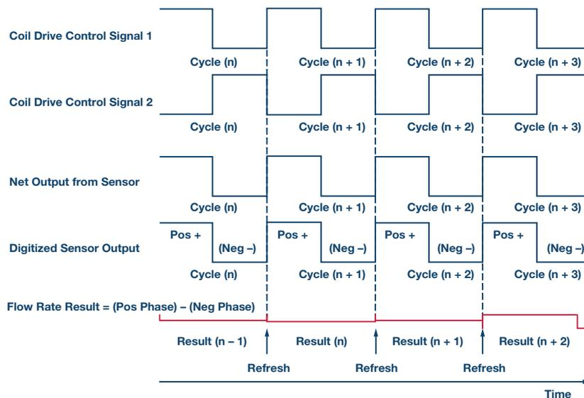
Figure 16. Synchronous demodulation and flow rate calculation in digital domain.
