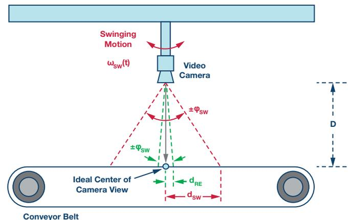
Figure 2. Industrial camera inspection system.
