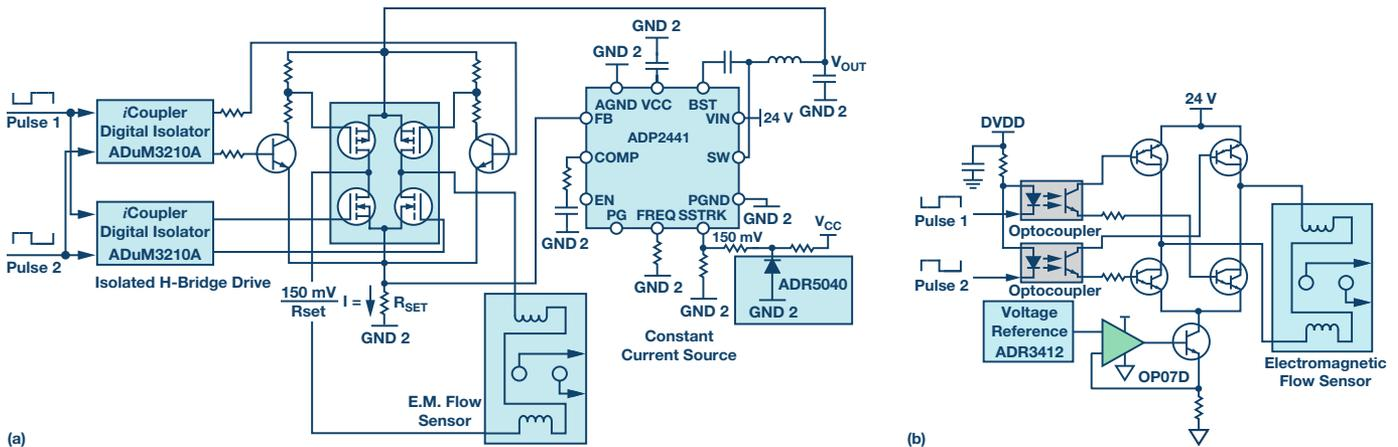
Figure 14. (a) Drive isolated H-bridge with SMPS and *iCoupler*.<sup>®</sup>
