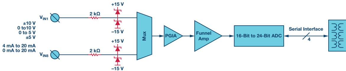
Figure 3. Discrete protection solution.
