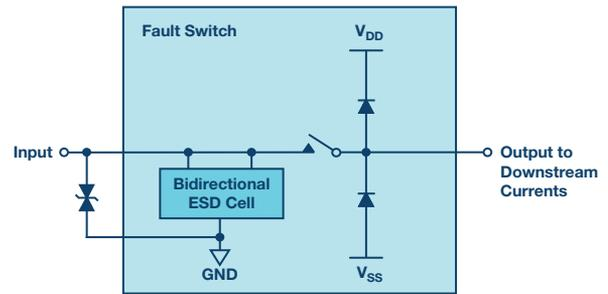
Figure 5. Fault protected switch architecture.
