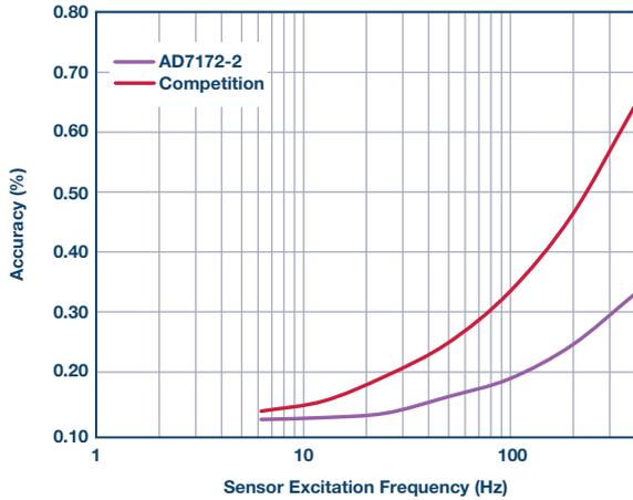
Figure 11. Comparison of measurement accuracy over sensor excitation frequency.
