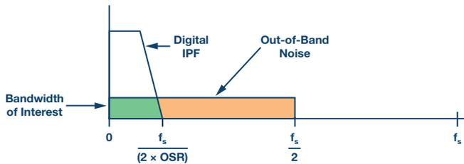
Figure 7. Oversampling of a Nyquist converter.
