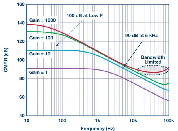
Figure 8. AD8220 dc and ac rejection of common-mode effects.
