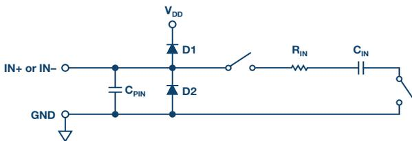
Figure 12. Equivalent analog input circuit.
