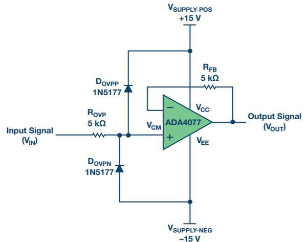
Figure 1. Classic clamping circuit for overvoltage protection.
