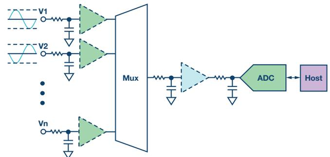
Figure 4. Multiplexed input signal chain.
