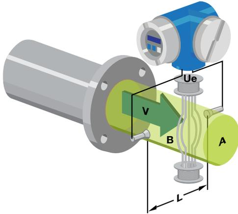
Figure 2. Working principle of the magnetic flow meter.
