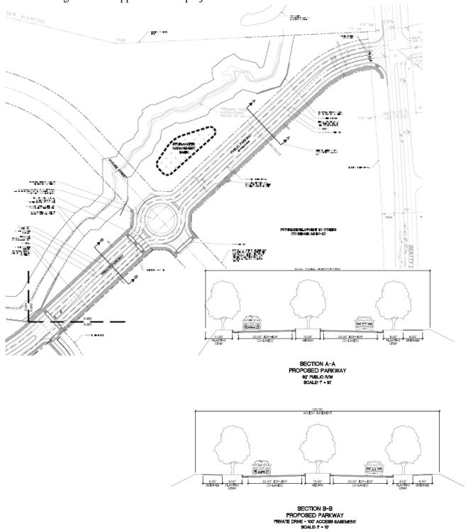
All new roads are required to be designed with curb, gutter, 8-foot wide sidewalk, a 6-foot wide landscape/street tree area, and travel lanes. The access parkway complies with city standards, except for a sidewalk segment on the north side of the parkway between Beatty Drive and the proposed traffic circle. The applicant is requesting relief from the required sidewalk within this segment due to:
