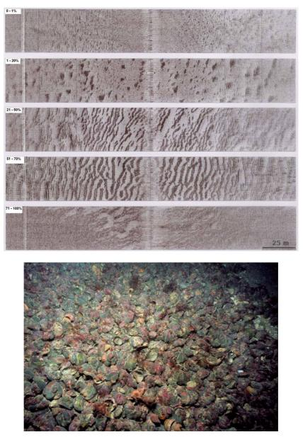
Fig. 2. Top: examples of sonograms showing several limpet covering rate levels (from 1, 20, 50, 70 to 100%). Bottom: Photograph (Ifremer) of a seafloor completely covered by the slipper limpet population.
