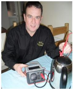
The results of testing are recorded in the instrument's internal memory and downloaded to the PATGuard 3 PC software program. In addition, images of visual inspections taken by the Apollo 600's onboard camera can also be transferred to the test records program.
