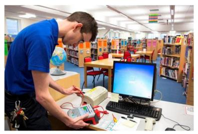
The focal point of the school's portable appliance testing policy is a Seaward Apollo 600 tester. This multi-purpose PAT tester combines electrical testing with sophisticated safety data collection features, including an onboard digital camera, to help those involved in maintaining safety in the workplace to demonstrate compliance with all the latest guidance on inspection and testing programmes.
