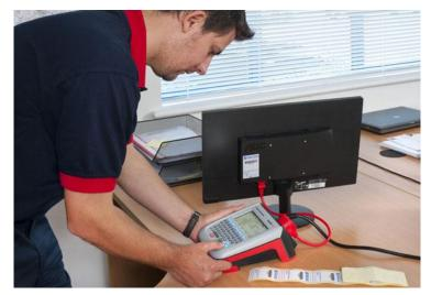
Code of Practice including, earth continuity, insulation resistance at 250V or 500V, protective conductor current, touch current, IEC lead polarity and RCD trip time.
