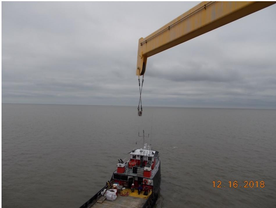
*Out of service crane from which the load block fell in close proximity to a nearby vessel.*
