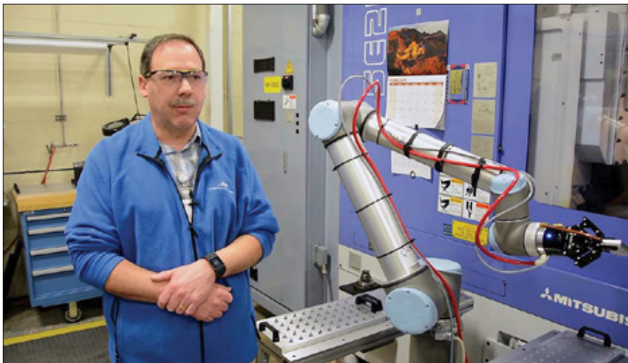
Customized grippers on this Universal Robots unit let Whippany Actuation Systems run two unattended shifts to meet increased production demand.
