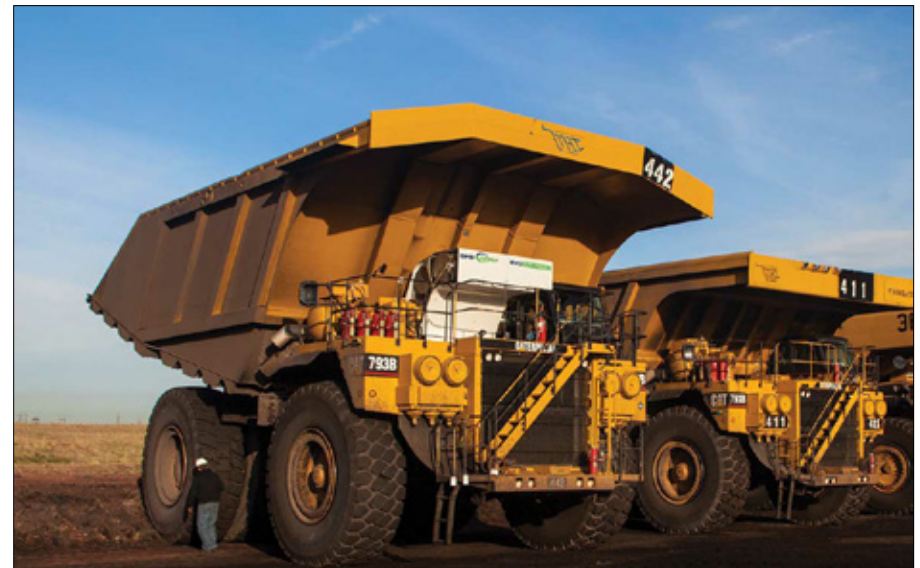
The GFS EVO-MT System for mine haul trucks provides an integrated, onboard LNG fuel storage system. The product BOM and design document control are managed by Arena PLM.
