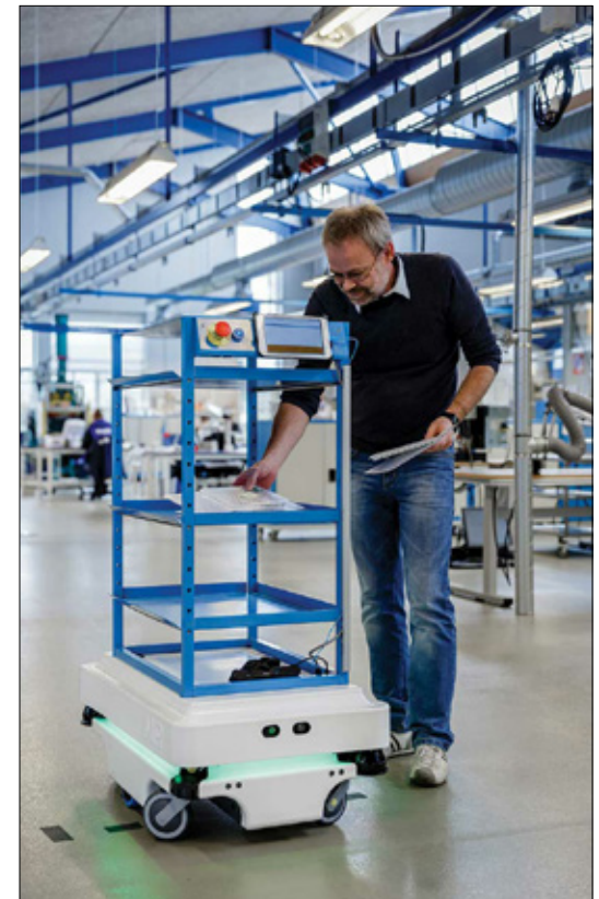
Self-driven mobile robots, such as this one from Mobile Industrial Robots, can avoid obstacles and change paths as they carry goods through a factory.
