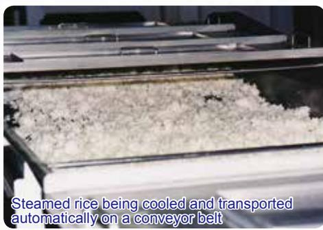
Steamed rice being cooled and transported automatically on a conveyor belt
