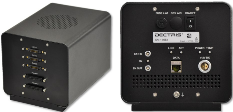
Figure 4.8: The PILATUS3 X CdTe 100K-M detector electronics unit viewed from the front (left) and back (right).
